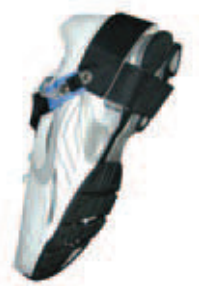
Figure 7. Heel grounder on an operator's shoe. These devices should be used with either an ESD floor or with grounded ESD mats placed at each work area. Photo courtesy of Transforming Technology Inc.
