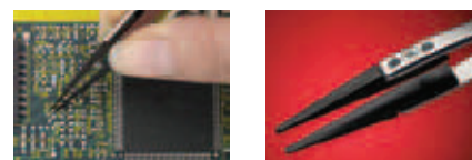
Figure 5. Tweezers with dissipative tips. Photograph courtesy of TDI, Inc.
